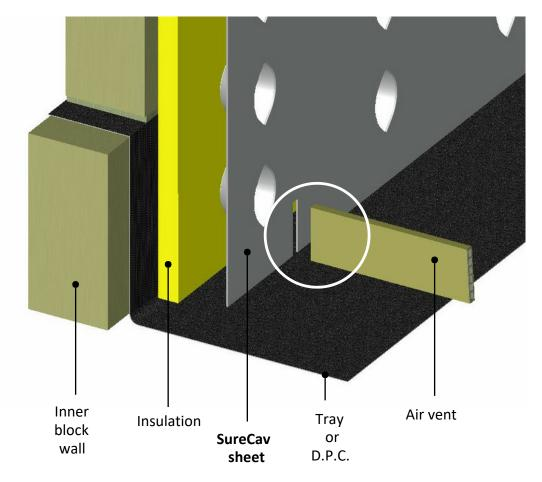
Cut a slot in the SureCav sheet 10mm wide and 65mm high to match the profile of the ventilator (as shown inside the white circle above). If the intended slot does not coincide with the edge of the SureCav sheet then simply drill a 10mm dia. hole at the top and bottom and cut the material away as shown on the right.
